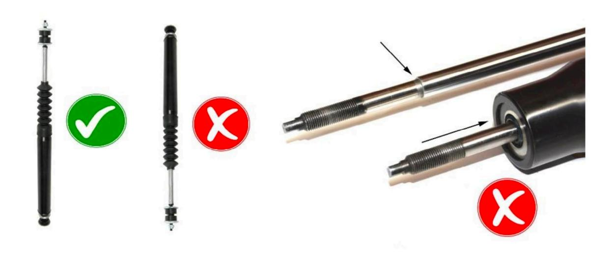
Before fitting the shock absorber, turn it the right way up (dust cover to the top), and operate it a few times by hand to prime the damper, taking care not to over-compress so that the lip on the operating shaft does not pass into the seal in the shock absorber body. If you over-compress the shock absorber it will not return and oil will leak past the seal, invalidating the warranty.
