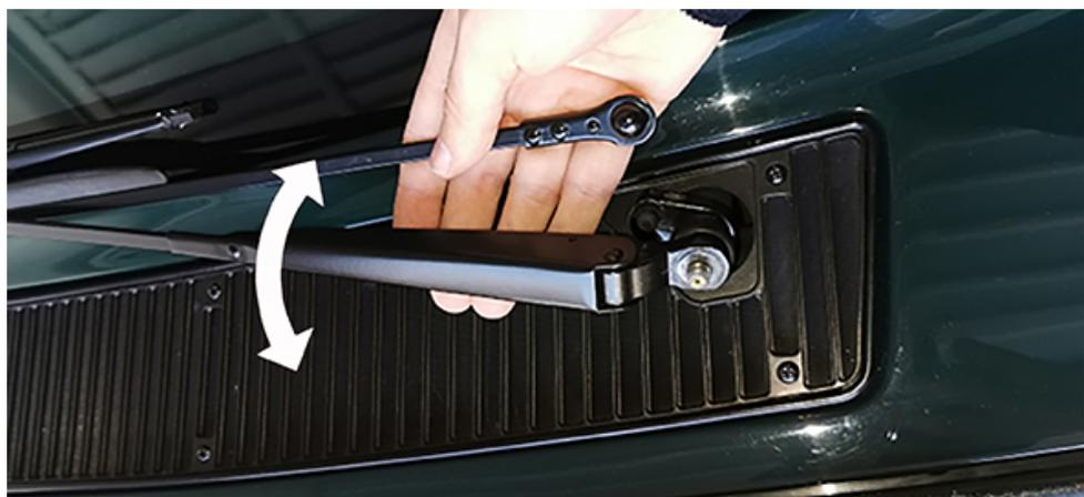
Manoeuvre and, once loose, remove the arm from the spindle.
