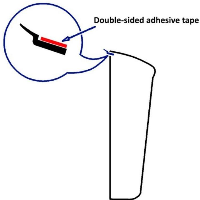
When the number plate mounting is tightened, the visible flap of the seal will follow the profile of the boot/trunk lid. *Please note: a gap is left at the along the bottom of the number plate mount to allow for the egress of any water that may accumulate.*
