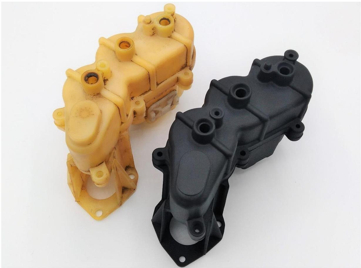
Figure 1: Seat Gear Box Casings. Left original, right reproduction unit
