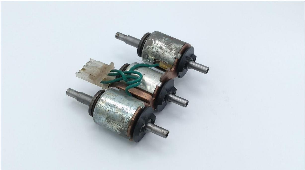
*Figure 5: Solenoid block with drive shafts and plastic clutches added*
