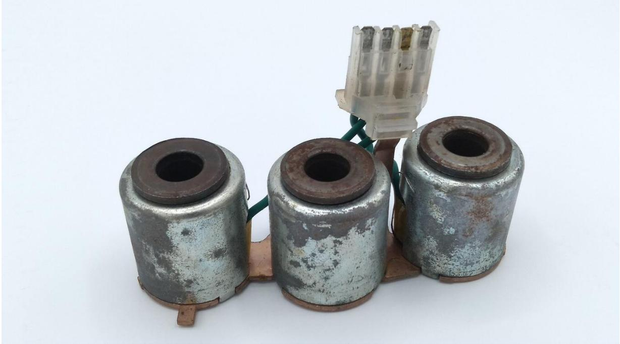
*Figure 4: Solenoids with sleeves inserted.*
