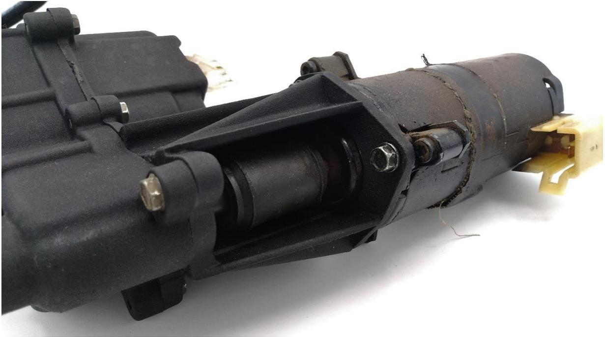
Figure 9: Assembled gearbox casing and motor
