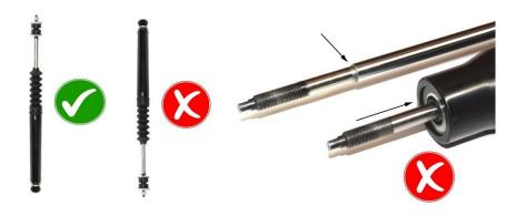
Before fitting the shock absorber, turn it the right way up (dust cover to the top), and operate it a few times by hand to prime the damper, taking care not to over-compress so that the lip on the operating shaft does not pass into the seal in the shock absorber body. If you over-compress the shock absorber it will not return and oil will leak past the seal, invalidating the warranty.
